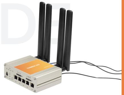
Unleash the power of 5G cellular connectivity and LTE fallback with the TOSIBOX® 695 - a game-changer for networking professionals! Crafted with precision and engineered for toughness, the TOSIBOX® 695 boasts a robust metal alloy casing complemented by an extensive temperature range and an IP30 Ingress Protection Rating. It's built to thrive in challenging environmental conditions.
