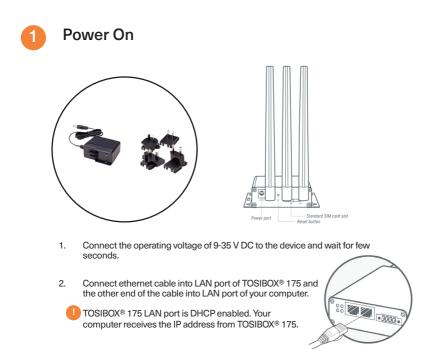
Plug the cable connecting to your computer into LAN port
